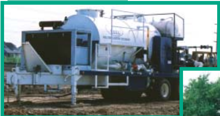
Specialized equipment injects the "Stabilizing Solution" under pressure into expansive materials in place.
